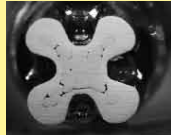
Crimp-cross section HARTING crimp profile
